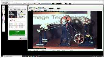
An Automated target tracking function allows for motion analysis of the image sequence. Vicasso supports Quadrant and spot targets and also will track any feature in the sequence.
